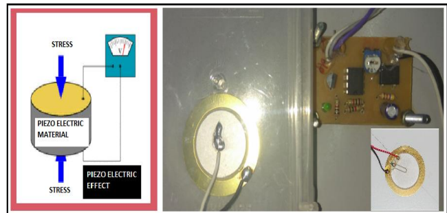
Fig4 Piezo Electric Effect & Piezo Sensor Circuit
